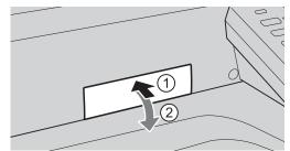
② Insert a PCMCIA/PC card into the PCMCIA/PC Card slot as illustrated. (Label side up)
